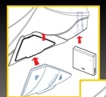
**SPEAKERS** and **MICROPHONE** are **PRE-INSTALLED** in your **SMART** helmet: just install the controller and the battery in the helmet, connect and enjoy!
